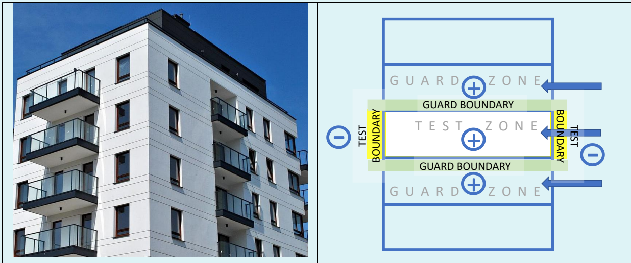
Figure 3: Schematic diagram of a guarded zone airtightness test
