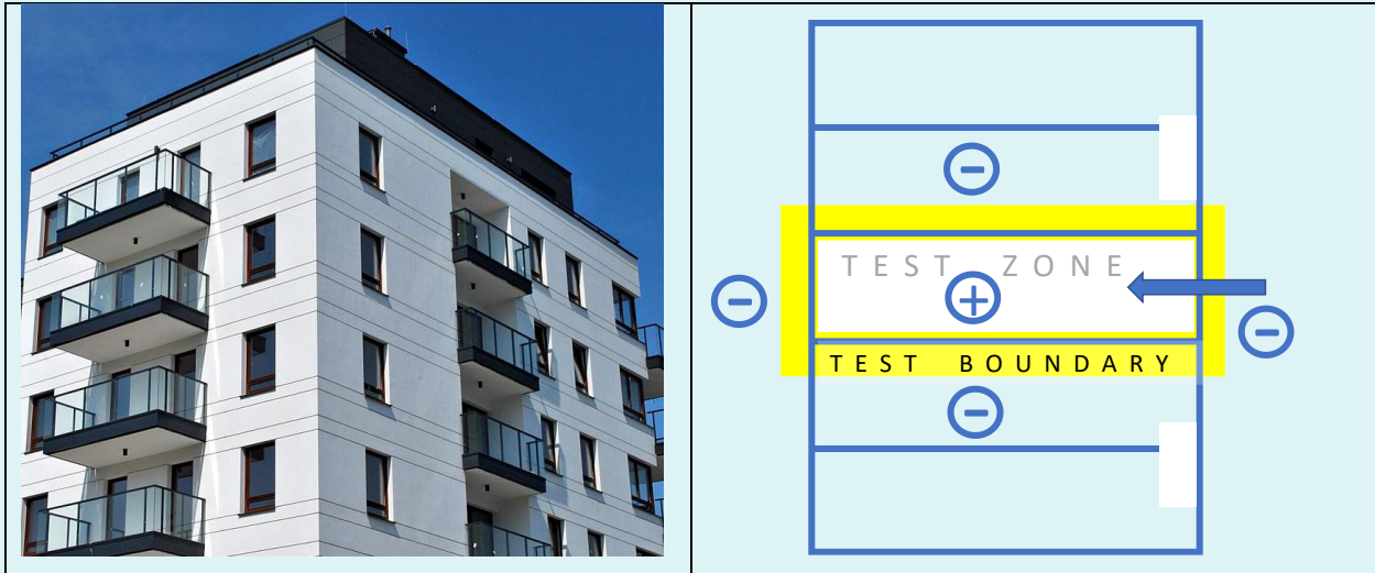
Figure 2: Schematic diagram of a zone airtightness test
